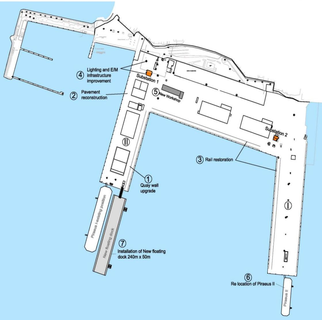
Installation of a **Panamax size floating dock** (80K dwt, 250m)
